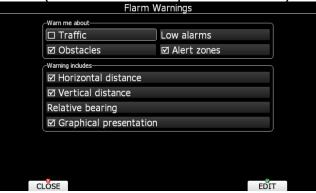
If the voice option is enabled it is also possible to hear the horizontal and vertical situation to the current object. Uncheck appropriate items if you want to disable this part of the message. You can also define the way direction to the Flarm object will be presented. There are three options:
