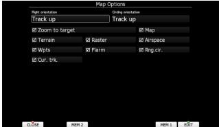
Map orientation is setup separately for straight flying or circling. If **Zoom to target** is checked the zoom will be automatically adjusted so that the target point is always visible. Maximum zoom is 200 km and minimum zoom is 1 km. The check boxes will turn on or off the following items:
