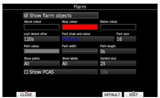
Checking **Show Flarm object** will enable display of aircraft detected by FLARM.
