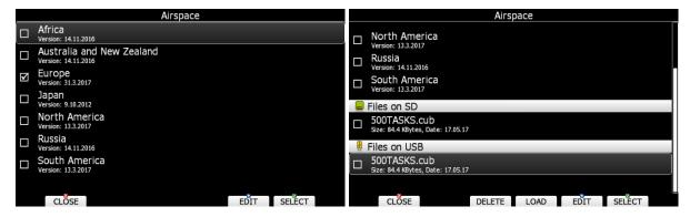
Select the required airspace and press **SELECT**. If a check mark is shown in front of an airspace item, this airspace file will be shown in the graphics and used for proximity calculation, when enabled.
