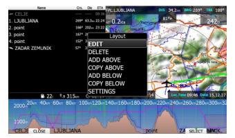
Pull down menu is used to select one of the options. Press button several times to select appropriate item of turn PAGE selector knob. Pull down menu will automatically close after few seconds.
