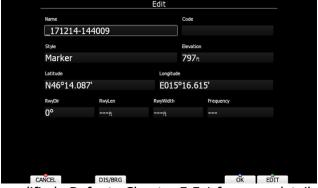
Waypoint data can be modified. Refer to Chapter 5.5.1 for more details. Press the **OK** button to save a marked waypoint or press **CANCEL** to exit without saving. Press **GOTO** button to navigate immediately to selected point.
