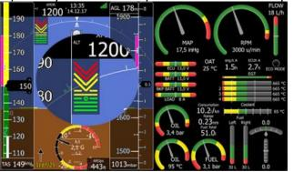
AoA symbol has three colours. Red colours indicates approaching to critical angles of attack (Stall), yellow indicates angles between minimum sink and best LD (lift over drag – gilde of the plane), green indicates angles of attack for cruise. Green circle indicates angle of attack, where aircraft has the best glide ratio.
