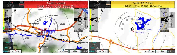
Picture above shows typical Flarm warning with graphical presentation and relative bearing of object. Press CLOSE to dismiss warning, CIRC.OFF to dismiss for time of circling and 1min to dismiss all Flarm warnings for one minute.
