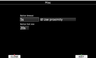
Screen button appearance can be set by **button timeout** time. Proximity will be detected after touch of a button if **Use proximity** is ticked. Also **button font size** can be set here.
