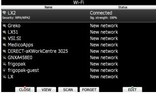
Press **SCAN** to scan for new networks. Use **EDIT** to enter password for selected network and to connect to it.
