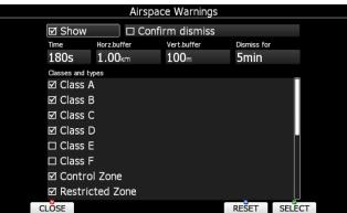
Airspace warnings are the most complex ones. An airspace warning is activated by two triggers; First warning (orange) will be given when a projected position of flight for period, which is defined in the **Time** item, is computed to cross an airspace zone.
