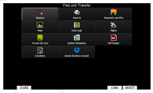
Within a profile user can selected different airport databases, airspace and waypoint files. Selected files can be stored inside main display unit or on inserted SD card or USB stick. It is also possible to upload files from SD card or USB stick to main display unit.
