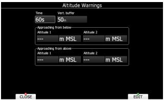
If the projected altitude is greater than the set altitude, an altitude warning will be raised. Projection is calculated based on the 20 second average vertical speed and time which is defined in the **Time** item. Altitude warnings will be raised in all modes and dialogues just as for airspace warnings.
