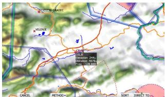
Details of selected airport will be drawn next to it. In upper-left corner of screen current sort method is shown. There are two possibilities, distance sort or bearing sort. Press **SORT** button to change it.
