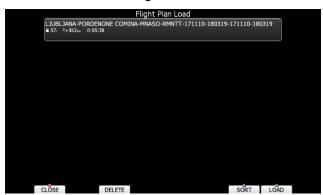
Total FPL distance, necessary fuel and required time are shown for each FPL stored. Select the desired FPL by rotating the PAGE selector knob and press **LOAD**. The FPL will be loaded into the active FPL and the FPL edit dialogue will be opened.
