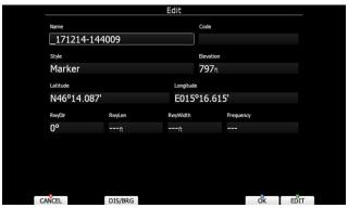
Waypoint data can be modified. Refer to Chapter 5.5.1 for more details. Press the **OK** button to save a marked waypoint or press **CANCEL** to exit without saving. Press **GOTO** button to navigate immediately to selected point.
