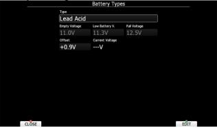
Use **Type** combo to select appropriate type of battery (Lead Acid, LiFe, LiPo, custom). You can see empty, low and full voltage for the selected type of battery. In case of voltage drop, because of cable lengths, you can set up voltage **offset** to adjust measurement of **current voltage**.
