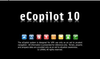
The boot procedure normally takes up to 20 seconds but in the case of a firmware update or system check it can take more time. The final boot screen displays information about the eCopilot system firmware and the serial number. When the boot procedure is completed the profile selection dialogue is shown. Please refer to Chapter 7.1 for more details about starting up the system.
