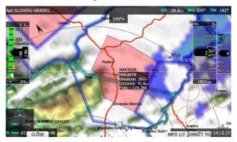
A blue cross will be plotted over the screen with info box for given cross position. Move cross up and down on map using PAGE selector knob. Move cross left and right using MODE selector knob. Turn ZOOM selector knob to zoom map.
