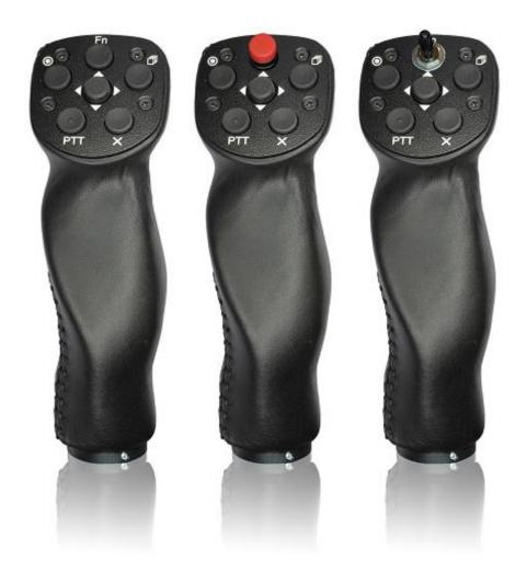
The stick is available also in various diameters: 18 mm, 19.3 mm, 20.3 mm, 24.4 mm and 25.4 mm. All necessary electronics is built into the top of the stick. The four coloured wires from the bottom must be connected to Remote CAN unit. Additionally one shielded cable is used for push to talk button.
