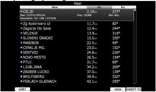
Press **VIEW** button to change how much details are visible for selected item. Select the preferred landable place via the PAGE selector knob and press the **DIRECT TO** button. It will automatically change to airport mode and navigation will commence to selected point. Duplicates are automatically removed. If a target with nearly the same latitude and longitude is found within both the distributed airports database and user waypoint file then only the
