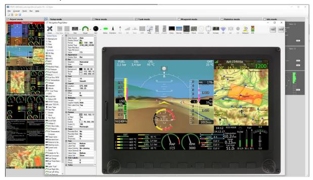
If new profile is created with LX Styler, it will have default device settings. However, it is possible to copy device settings from profile to another profile. Select newly created profile as active profile. Select profile from which you would like to copy settings to active profile. Press **COPY** button. A confirmation dialog will open.
