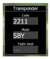
Use **MODE** to select mode of operation of connected transponder (**STBY, GND, ON, ALT**). Press **CODE** to enter squawk code. Press VFR to automatically set squawk code to 7000. Press **IDENT** to identify.
