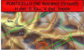
An Airspace warning will be raised in all modes and dialogues. A warning for an alarmed zone can be dismissed for a whole day, some minutes or just quit. **Quit** means that the message will disappear. Use **Dismiss for** spin to define dismiss time in minutes. This time will be
