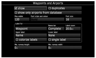
The **Max.visible** item defines how long waypoint labels and detailed symbols are shown. If the maximum number of waypoints on the current screen is more than the defined value only small blue dots will be shown for waypoints and no labels will be drawn.
