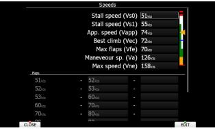
Once speed range is entered, the system will be able to display requested flap position based on current wing loading and g-factor.
