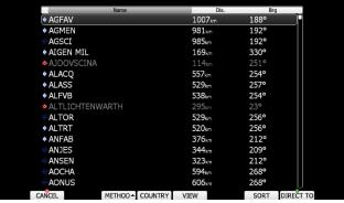
Press the **VIEW** button to change details of selected airport. Press the **SORT** button to change the sort order of the airports. Select an airport using the PAGE selector knob. Press
