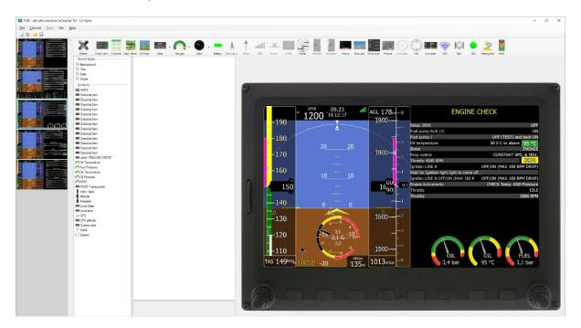
Press save to save the checklist file on the PC/SD card or USB. File has the extension .checklists
