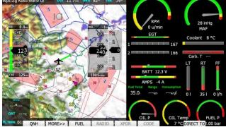
Press the **MORE>>** button to see more options. If the remote stick is available the behaviour is slightly different. When the check button is pressed on the remote stick a menu will appear instead of the button functions.
