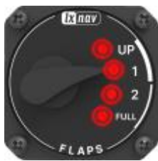
No communication with the flap controller
