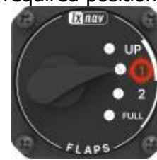
Flap didn't reach the required position 1
